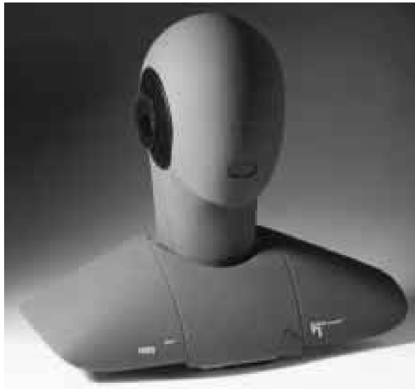
Figure 1 Artificial head measurement system with mathematically definable geometry, calibratable transmission characteristics and built-in equalizers [2]
