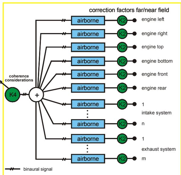
**Figure 3.** Binaural synthesis based on airborne and structure-borne sound transfer paths
