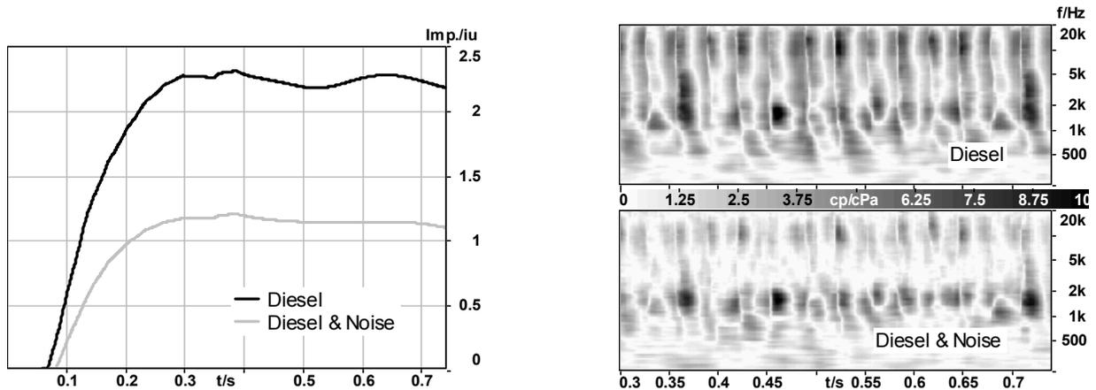
**Figure 1.** *Impulsiveness based on the Hearing Model according to [2] (left) and detection of significant time and frequency patterns using the “Relative Approach Analysis” (right) of a diesel noise and of the same signal with additional noise*
