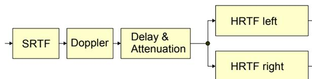
**Figure 4.** *Simulation model of pass-by noise for one single path [7]*
