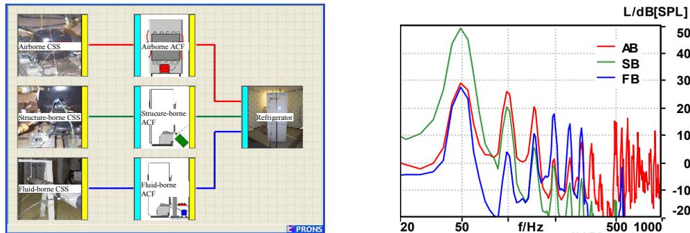
**Figure 6.** PRONS model of a refrigerator (left) and corresponding predicted spectra (right)
