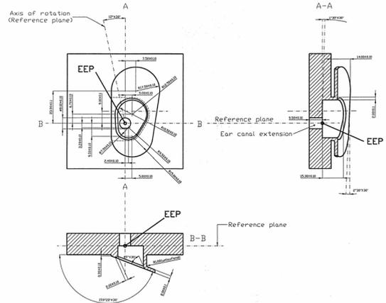
Fig. 6: Artificial ear, type 3.4, ITU-T P.57
