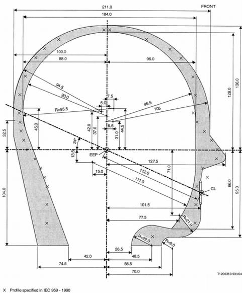
Fig. 5: Limits of the head cross-section in the vertical plane – dimensions in mm, ITU-T P.58
