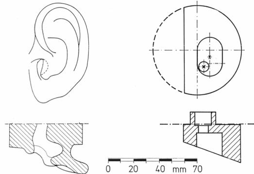
Fig. 3: Pinna with a simplified mathematical describable external geometry, reduced to the dimensions important for the directional pattern of the external ear transfer function
